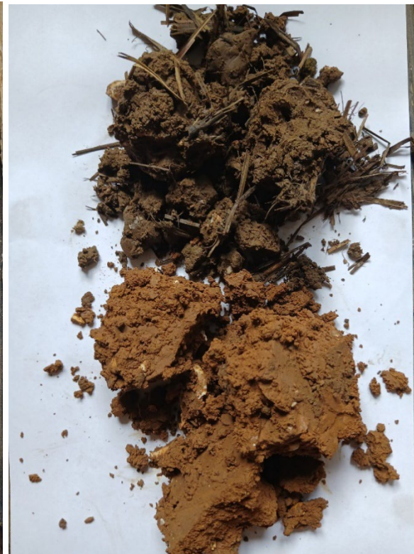
Graphic A-3 3F3602HP Medium clay loam over slowly permeable clay. WC IV and Subgrade 3b
