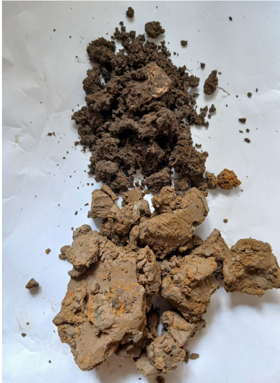
Graphic A-7 3L6027HP Typical Windsor soil. Clay/silty clay over clay. WC IV and Grade 4
